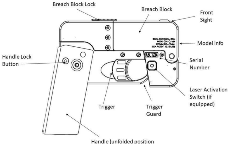
To unfold the IC9mm into a shooting position, first ensure that the muzzle of the firearm is always pointed in a safe direction. Next, grip and rotate the handle away from the body of the firearm, as shown in the images above. When fully extended, the handle will lock in place. Confirm that the handle is fully open and locked into place prior to loading, unloading, or firing the IC9mm.
