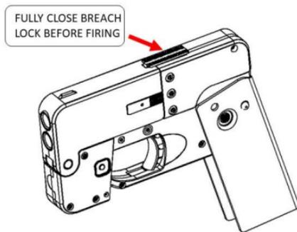
Never load or unload the firearm inside a vehicle, a building, or any other enclosed space (except in a designated firing range). Before loading the firearm, wipe away any excess grease or foreign substance, and visually confirm that there are no objects or other materials inside the barrel or internal breach block area.
