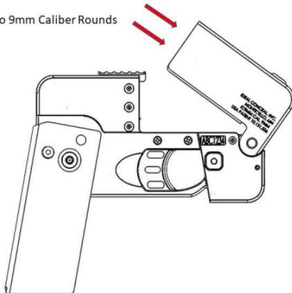
(iii) Close Breach Block Latch
