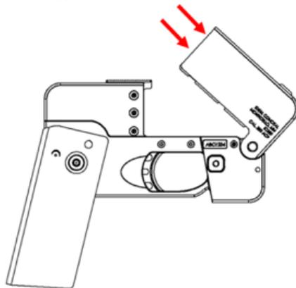
(iii) Close Breach Block Latch
