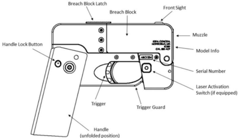
To unfold the IC380 into a shooting position, first ensure that the muzzle of the firearm is always pointed in a safe direction. Next, grip and rotate the handle away from the body of the firearm, as shown in the images above. When fully extended, the handle will lock in place. Confirm that the handle is fully open and locked into place prior to loading, unloading, or firing the IC380.
