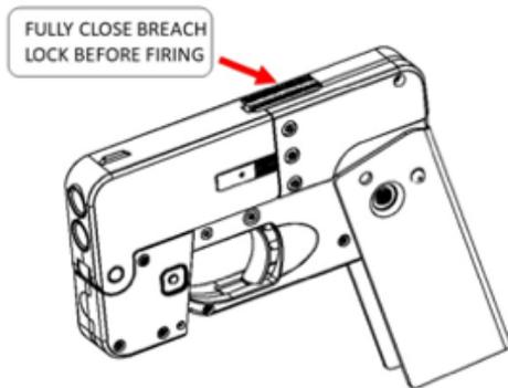
breach block into a closed position, as shown in the image above. Always be certain that the breach barrel latch is fully closed and engaged before firing.
